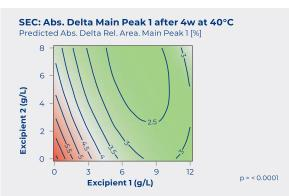
We stabilized a bispecific antibody via optimization DoE at accelerated aging temperature. The contour plot shows the predicted sweet spot in the excipient design space corresponding to the smallest loss of the main peak by SE-HPLC. This allows refining the concentration selection for the best formulation candidate.
